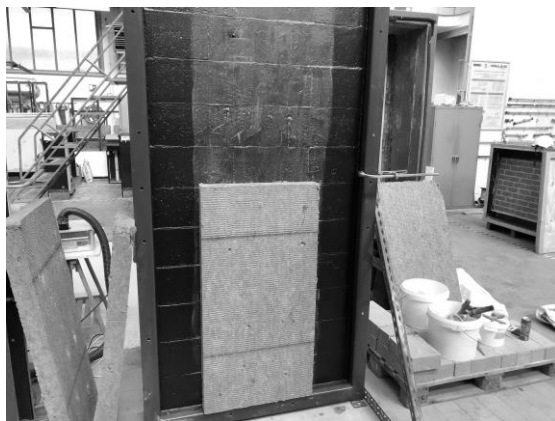
Figure 9: Insulation panel placed on the walls
