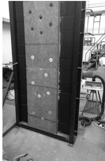
Figures 14: Concrete walls with PASSIVE PURPLE (left) and PASSIVE PURPLE EXTERNAL (right), PRIMER 52, REDArt™ CAPA BASE CASA, ROCKWOOL® ROCKSATE DUO PLUS and 15 anchors (6 green Ejot H2, 6 white Ejotherm STR U 2G, 3 grey Rawlplug®)
