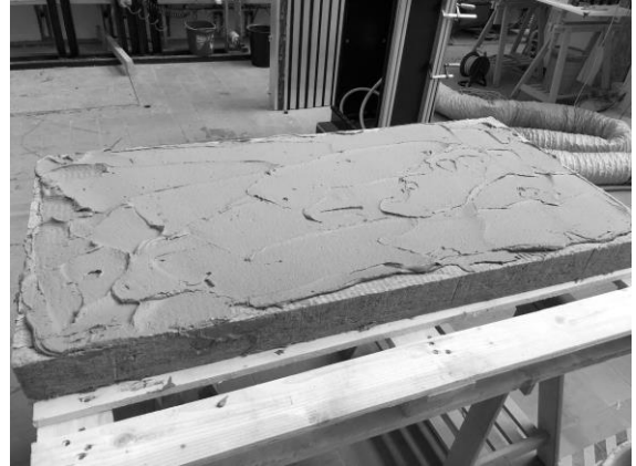
Figure 8: Insulation panel covered with mortar REDArt™ CAPA BASE CASA
