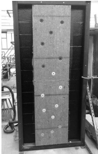
Figures 14: Concrete walls with PASSIVE PURPLE (left) and PASSIVE PURPLE EXTERNAL (right), PRIMER 52, REDArt™ CAPA BASE CASA, ROCKWOOL® ROCKSATE DUO PLUS and 15 anchors (6 green Ejot H2, 6 white Ejotherm STR U 2G, 3 grey Rawlplug®)
