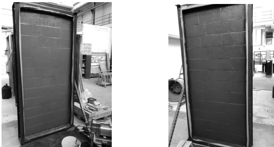
Figures 3: Walls covered with PASSIVE PURPLE (left) and PASSIVE PURPLE EXTERNAL (right)
