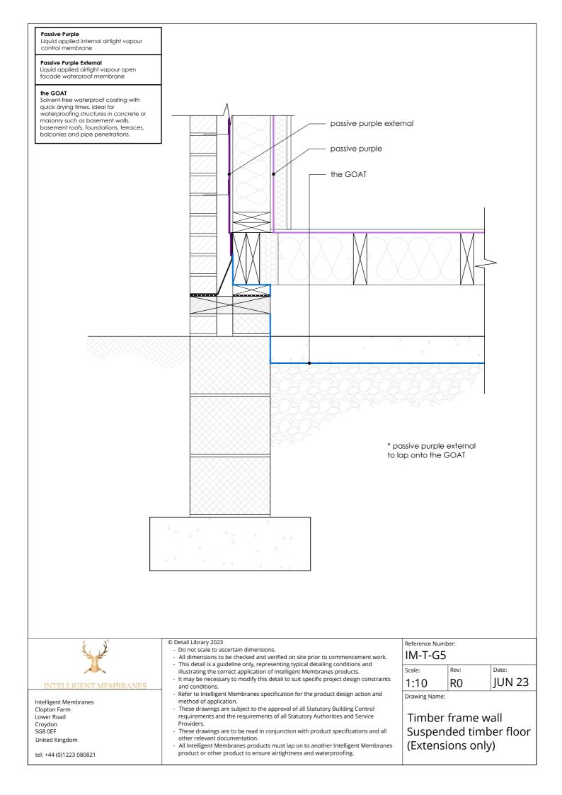
Liquid applied internal airtight vapour control membrane
