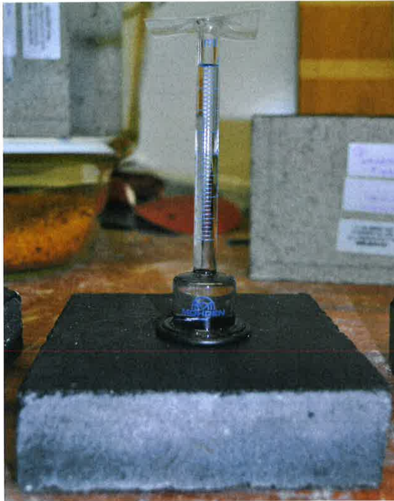
Figure 2 – Water absorption test
