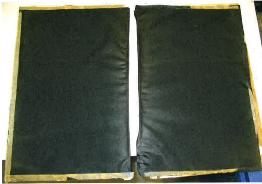
Figure 2 – Sheets of PASSIVE PURPLE EXTERNAL after exposure to UV-radiations
