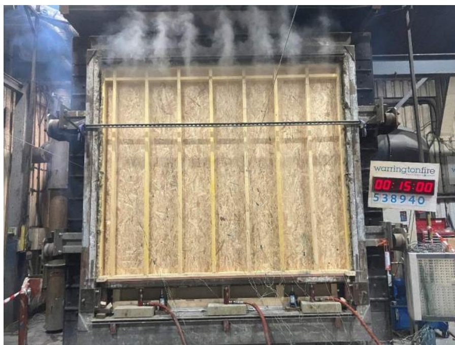
Figure 20 Unexposed face of the specimen after 15:00 minutes of testing
