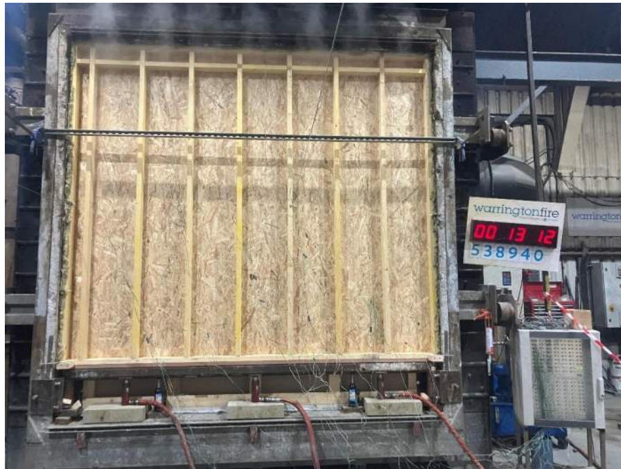
Figure 19 Unexposed face of the specimen after 13:12 minutes of testing
