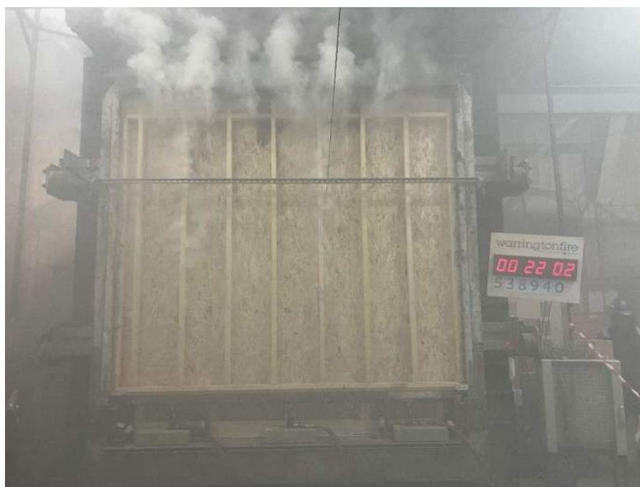
Figure 22 Unexposed face of the specimen after 22:02 minutes of testing
