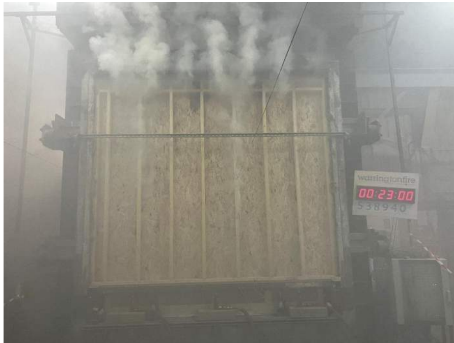
Figure 23 Unexposed face of the specimen after 23:00 minutes of testing
