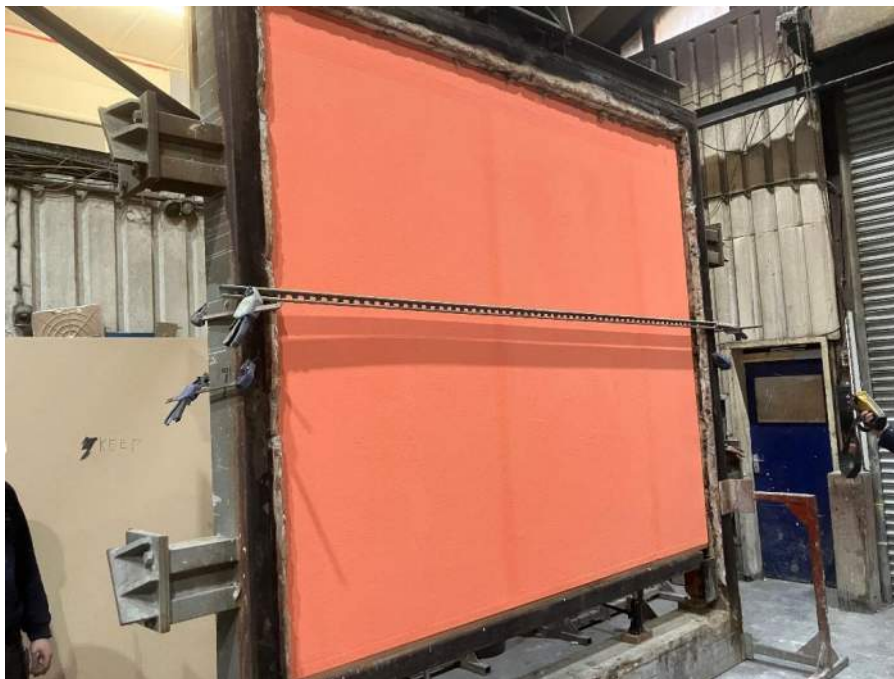
Figure 18 Exposed face of the specimen before the start of the test (support bar and clamp removed prior to fitting onto furnace as well as the addition of fire stopping around the vertical edges and head)
