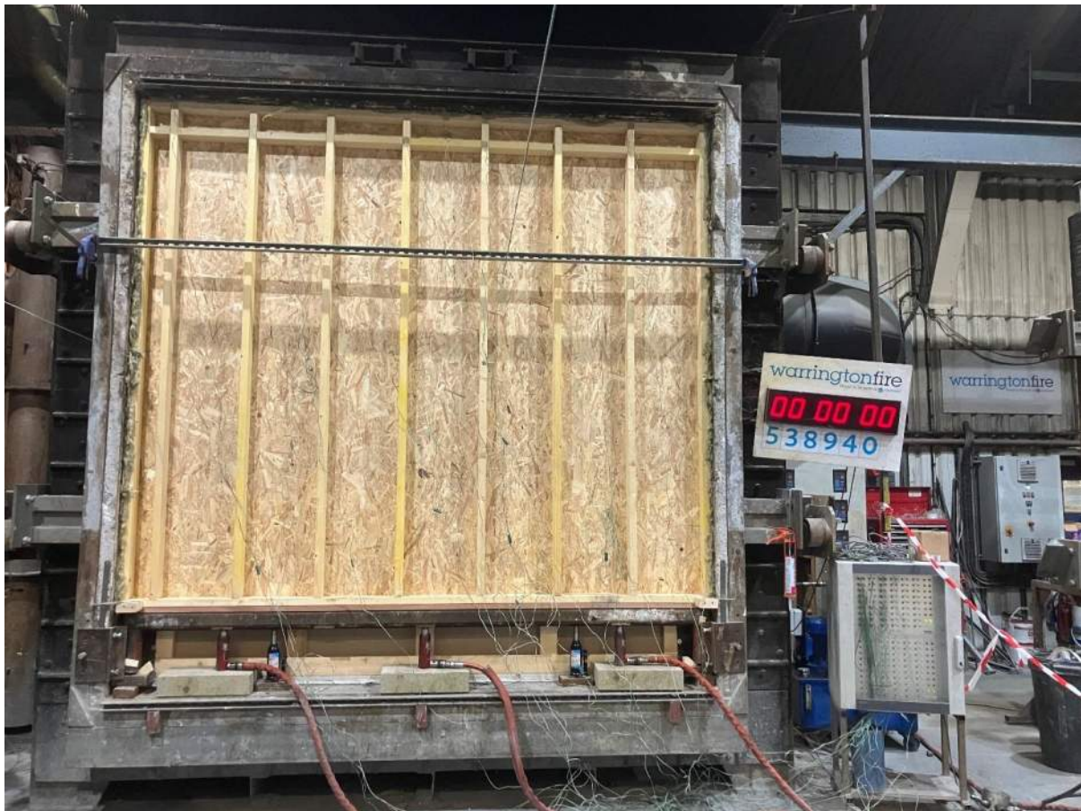
Figure 1 Unexposed face photograph of test construction
