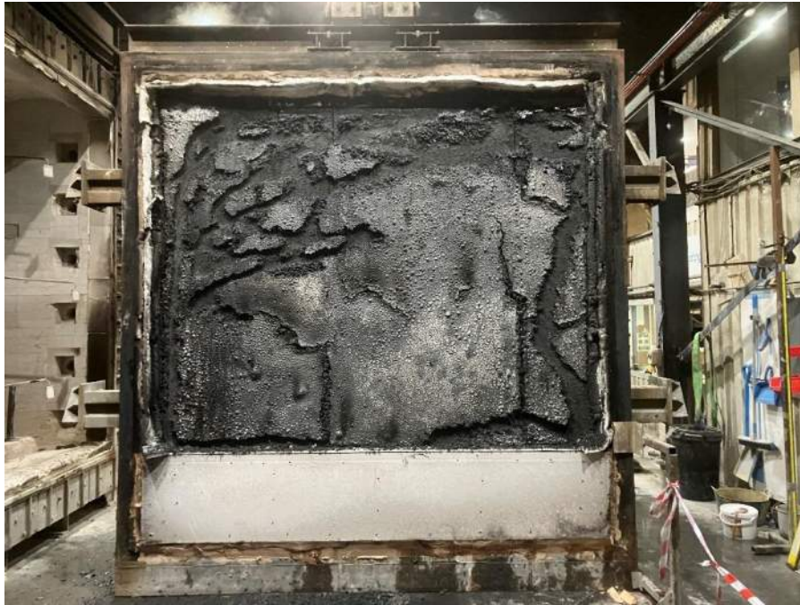
Figure 25 Exposed face of the specimen after the test
