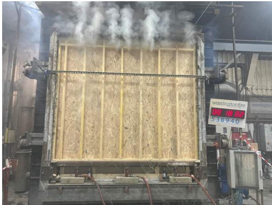
Figure 21 Unexposed face of the specimen after 18:02 minutes of testing
