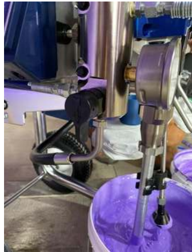
St max 2 pro 595 HI boy airless spray machine or similar in process
